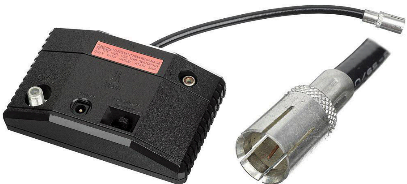
Fig. 6 - The Atari Switchbox, the automatic TV switch (photo: Evan-Amos - source: Wikimedia Commons)
