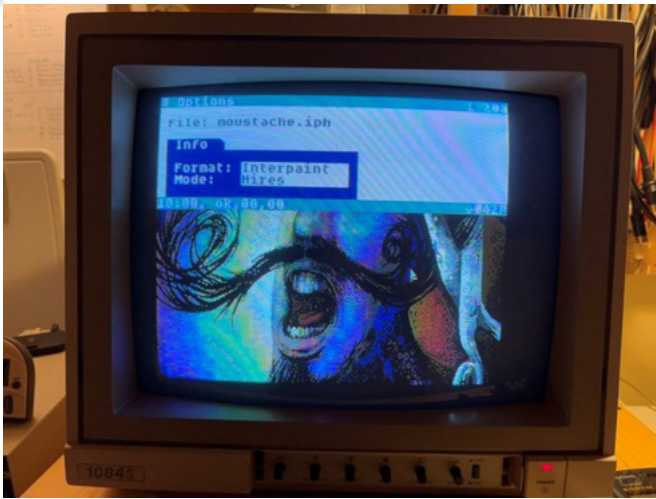
Fig. 4 - Embedded within the OS is the viewer to display the most common image file formats
