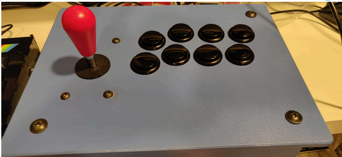
Fig. 12 - USB arcade joystick with zero delay controller used to test the console
