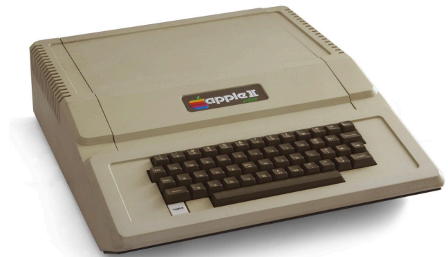
Fig.5 - An Apple II+. Apple II models are equipped with the 6502 (photo by Bilby)
