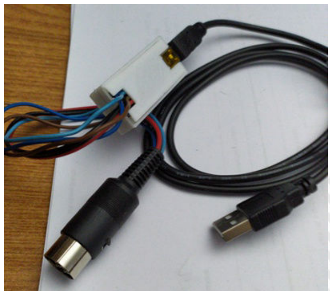
Fig. 9 - The UNO2IEC cable with its protective case
