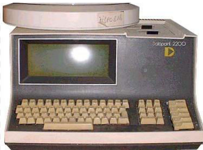
Figure 1: Datapoint 2200: its CPU consisted of 100 7400 series integrators (photo: Wikimedia Commons)
